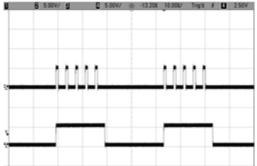
**Inhibit Mode** – Channel H is used to inhibit the output of the selected channel(s). This is an active high pulse, thus when channel H is high the selected channel(s) will **NOT** output pulses.
