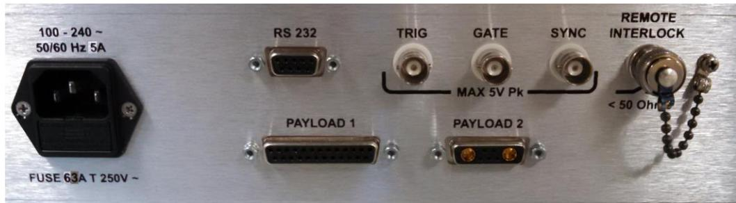
Figure 20 Power Supply Connections (Payload2 not installed)
