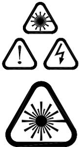
**Caution labels, in accordance with CDRH and CE requirements, are prominently displayed on the Laser Optical Assembly and Laser Power Supply. The maximum ratings indicated on the system labels are in excess of the normal operating parameters. Please refer to the Data Summary Sheet for specific information pertaining to your system.**
