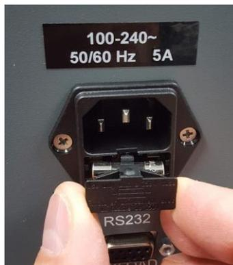
4. Remove the fuse and replace with a fuse with the following specifications: 6.3A, 250VAC, 5mm x 20mm Slow Blow.
